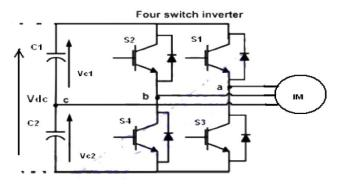
Fig(2.) FSTPI with Induction Motor
